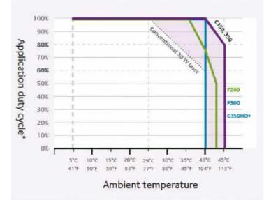
By contrast, many competitor laser coders can only operate effectively at up to 40°C with application duty cycles limited to a maximum of 60% as they only have a single fan at the end of the laser and insufficient scanhead cooling. Indeed, Markem-Imaje's advanced **Intelli'Cool**® systems mean manufacturers can replace less efficient, cumbersome higher wattage laser coders which require mandatory water cooling above 35°C.
