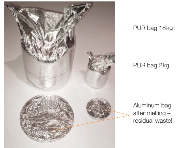
The bag content is completely molten. No loss of adhesive!
